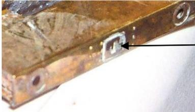
Buffer beam reinforcing plates
