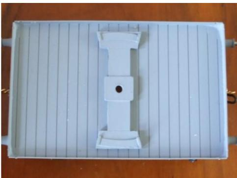
12. Glue the bolster support plate casting (Part 15) into position, it needs to line up with the fit into the holes situated in the top and halfway along the chassis.
