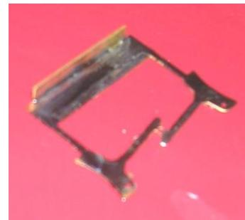
4. Place the brake gear assembly against the inside of sole-bar and slide down the chassis until the hole in the 'V' hanger and the hole in the brakes line up. And solder in position as shown.
