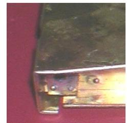
6. Next remove the buffer beam reinforcing plates (Part 5) and punch out the half etched rivets and tin the back of each piece with 188C solder. Now sweat the plates onto the half etched square in the front of the buffer beam.
