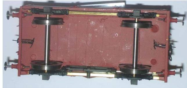
8. Punch out the half-etched rivets on the outside V-hanger (part13), fold up, and glue into position on the sole-bar and to the spigot of the brake gear casting. Repeat for the other side of the wagon.
