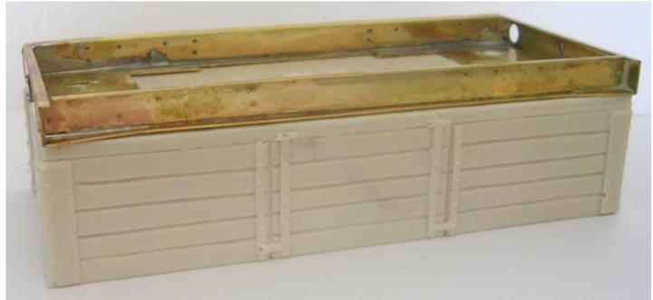
2. Next remove the 'L' section bars from the etch (parts 5) and punch out the half etched rivets as shown. There are eight 'L' sections with this kit. If you are building the E&WYUR wagon then you will need 'T's on the ends of the wagon. However if you are building the LD&ECR you have a choice of fitting 'L's or 'T's. Please note that the 'L's are handed and you will need a right and a left handed 'L' for each end of the wagon. The 'T's are made up from two 'L's placed back to back. As shown.
