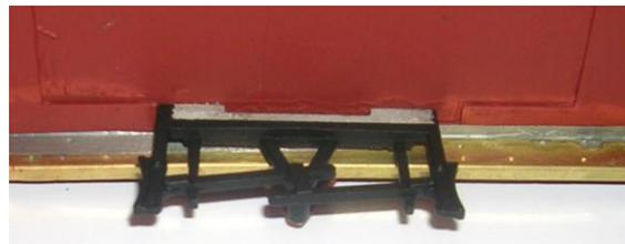
6. Drill out the w-iron castings to suit the bearings of your chosen wheels. Assemble a wheel set, 2 x W-iron's (part 12), 2 x bearing's and 1 x wheel/axle unit,
