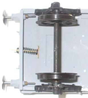
4. Drill out the w-iron castings to suit the bearings of your chosen wheels. Assemble a wheel set, 2 x W-iron's (part 10), 2 x bearing's and 1 x wheel/axle unit, do not glue the bearings into the W-irons at this stage. Again using two part epoxy resin, glue the
