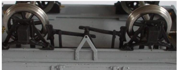
7. Next fold up and fix the out side Brake 'V' hanger to the sole bar lining up with the brake gear casting as shown.
