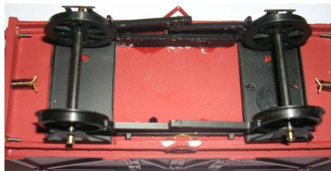
Glue the brake gear into position using two part epoxy resin, this will give you opportunity for adjustment. Position the casting with care centrally between the rivets on the sole-bar. Repeat the procedure for the opposite side.
