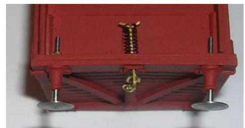
8. Next fold up the brass w-irons (Part 11-12) and rocking plate (Part 13). Slot the tags on the rocking plate through the slots on the w-iron that with the circles in the base and then twist round to secure.
