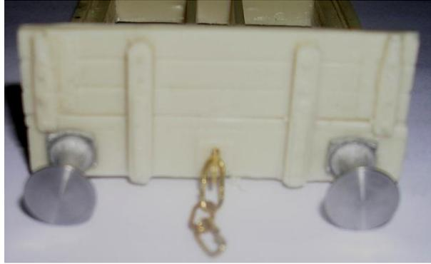
back of the coupling hook and bend the tags over to secure the spring in place. Then fix the four buffers (part 5) into the cast buffer plates (part 6) and then into the holes in the buffer beam using two part epoxy as shown. Repeat for the other end.
