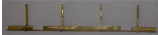
8. Next, fit the running boards to the sole bars of the model as shown. You are now ready to paint the model in the livery of your choice.
