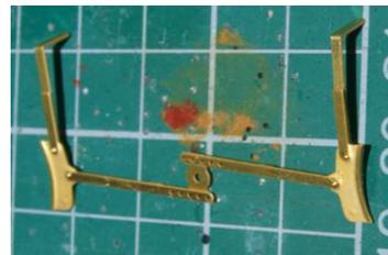
9. Attach the "V" hangers (part 11) to either side of the sole bar and then attach the brake blocks to the inside of the sole-bar as
