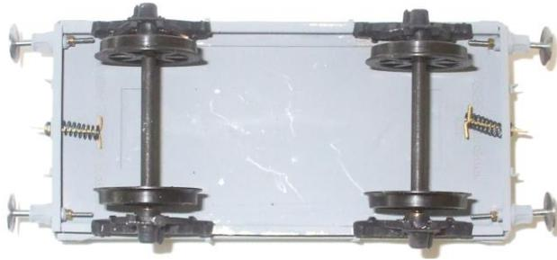
4. Next laminate the brake blocks together these are made up from one central blank (parts 12) and 2 brake shoe (part 13) parts.
