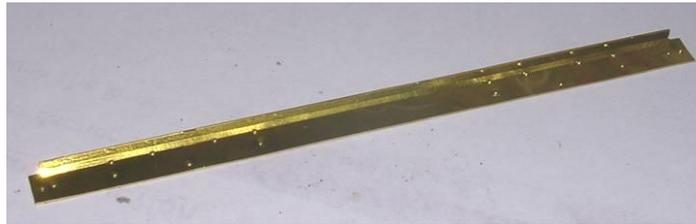
4. Click one of the sole-bars in to the half etch slot that runs between the two buffer beams and the rivets are facing out.. Solder into position using 188C solder. Make sure that the sole-bars are actually soldered inside the buffer beam. Repeat for the other sole-bar.
