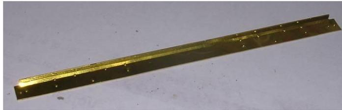
4. Click one of the sole-bars in to the half etch slot that runs between the two buffer beams. Solder into position using 188C solder. Make sure that the sole-bars are actually soldered inside the buffer beam. Repeat for the other sole-bar.
