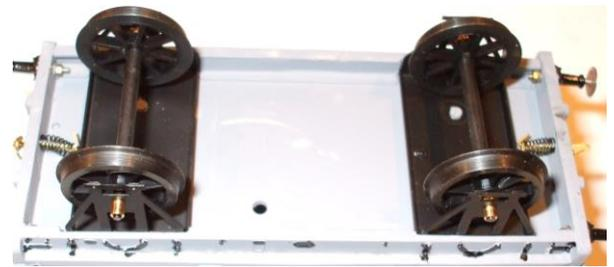
10. Place the brake gear casting (part 13) against the inside of sole-bar and slide down into the chassis with the spigot pointing outward. You may require to chamfer the casting so that it clears the filet between the
