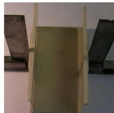
4. Then fit the ends (Parts 4) again make sure that the ends line up and are square.
