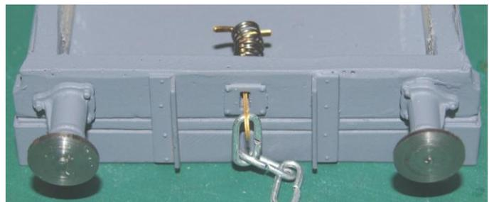
over the back of the back of the coupling hook and bend the tags over to secure the spring in place. Repeat for the other hook. Now fix the four buffers (part 9) then into the holes in the buffer beam using two part epoxy, as shown. Repeat for the other end.
