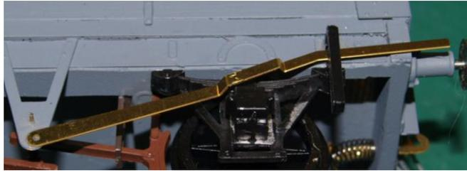
12. Next if you are building the diagram 32A bolster you will need to drill out the bolster (part 16) so you can fit the bolster pivot (part 17) and the wire.
