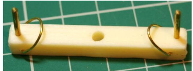
14. Next fit the bolster onto the pivot plate then fit to the assembly onto the wagon centrally.
