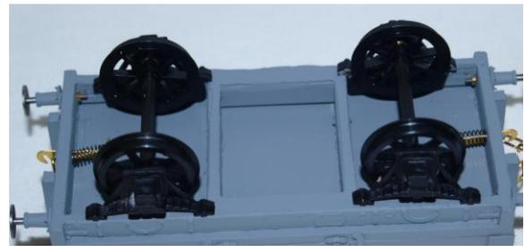
9. Glue the brake gear (part 11/12) together onto only the one side of the wagon, as shown. Then glue the outside V-hangers (part 13), into position on the sole-bar and to the spigot of the brake gear casting.
