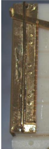
9. Punch out the half etched rivets and fit the brake ratchets (part 11) and fix into the half etched recesses on the end.
