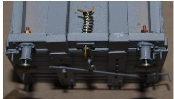
Fix the four buffers (part 16) into the holes in the buffer beam using two part epoxy.
