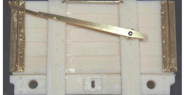
10. Fold up the brake lever (part 12) then attach it and the brake lever reinforcing plate using a pin, as shown. Then fold up some of the wire in to hand rails which fit into the holes previously drilled.
