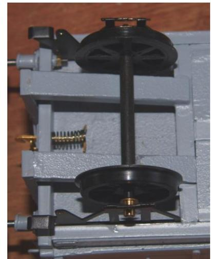
glue the assembled wheel set onto the sole-bars so that they are square and line up with the rivets as shown in the drawing.
