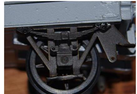
15. Next laminate the brake blocks together these are made up from one central blank (parts 20/21) and 2 brake shoe (part 22) parts.
