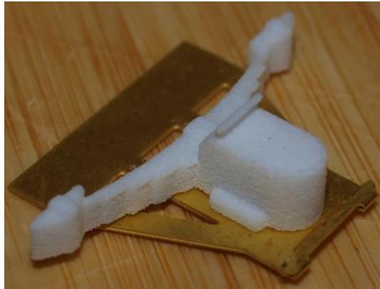
the W-irons. Again using two-part epoxy resin, glue the assembled wheel set onto the sole-bars so that they are square and line up with the rivets as shown on the drawing.
