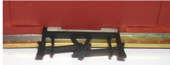
6. Drill out the w-iron castings to suit the bearings of your chosen wheels. Assemble a wheel set, 2 x W-iron's (part 12), 2 x bearing's and 1 x wheel/axle unit, do not glue the bearings into the W-irons at this stage. Again using two part epoxy resin, glue the assembled wheel set onto the sole-bars so that they are square and line up with the rivets as shown in the drawing.
