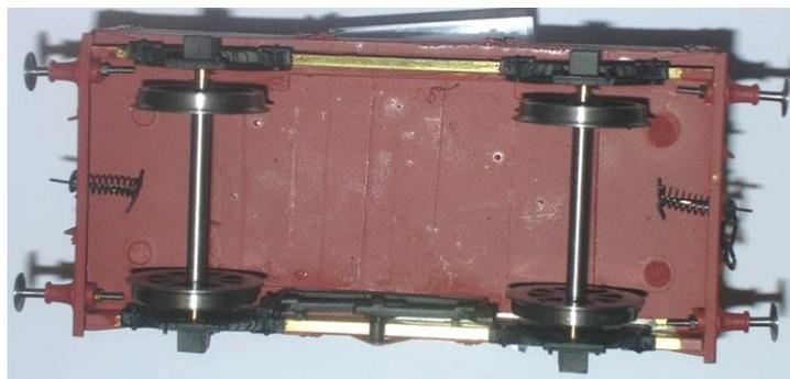
8. Punch out the half-etched rivets on the outside V-hanger (part13), fold up, and glue into position on the sole-bar and to the spigot of the brake gear casting.
