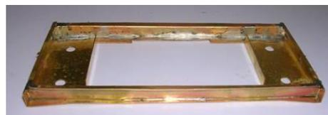
5. Next remove the buffer beam reinforcing plates (part 3) and punch out the half etched rivets and tin the back of each piece with 188C solder. Now sweat the plates onto the half etched square in the front of the buffer beam, as in photo.
