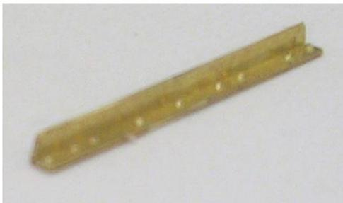
3. Next remove the Angle 'L' section bars from the etch (parts 6) and punch out the half etched rivets then fold. Now attach two of the Angle
