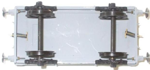
5. Next laminate the brake blocks together these are made up from one central blank (parts 11) and 2 brake shoe (part 12) parts.
