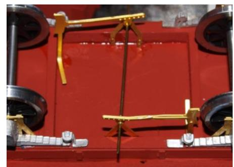
15. Next fix the brake lever (Part 15) and ratchet casting (part 16) to the sole-bar and to the outside of the 'V' hanger as shown.
