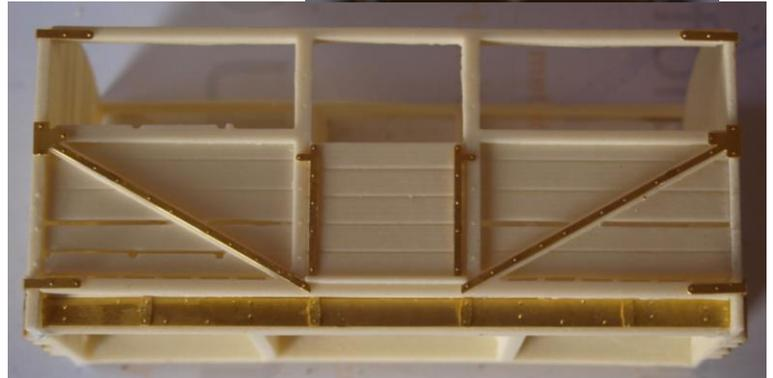
9. Next fit the wire into the hole that you previously drilled in the sides and ends
