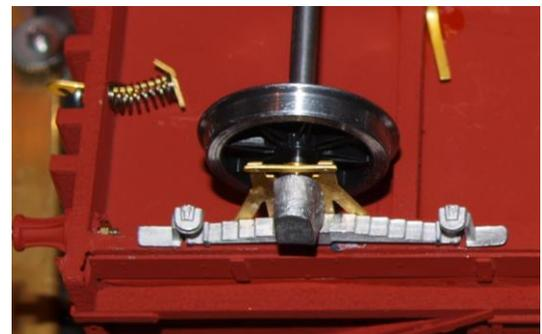
14. Next take the etched brakes (part 13) punch out the rivets and solder together. These can then be mounted on to the chassis next the wheel as shown. Using the etched 'V' hangers (part 14) against the bottom of sole-bar and next to link arm of the etched brake assembly. Glue the casting into position using two part epoxy resin, this will give you opportunity for adjustment.
