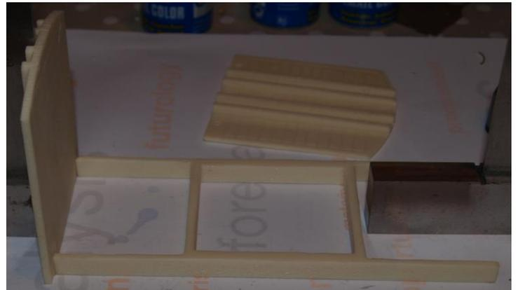
6. Then fit the floor (Parts 4) again make sure that it fits between the sides and ends. This is large and will need trimming to fit.
