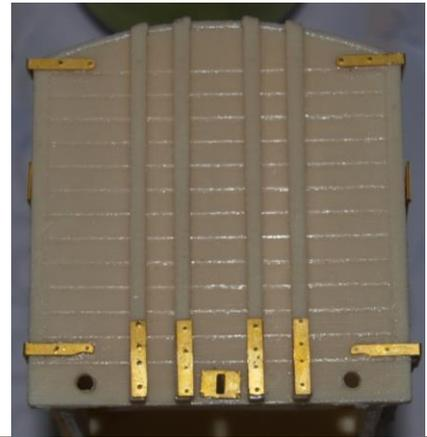
8. Next punch out the rivets on the sole bar etch (part 7) and attach.
