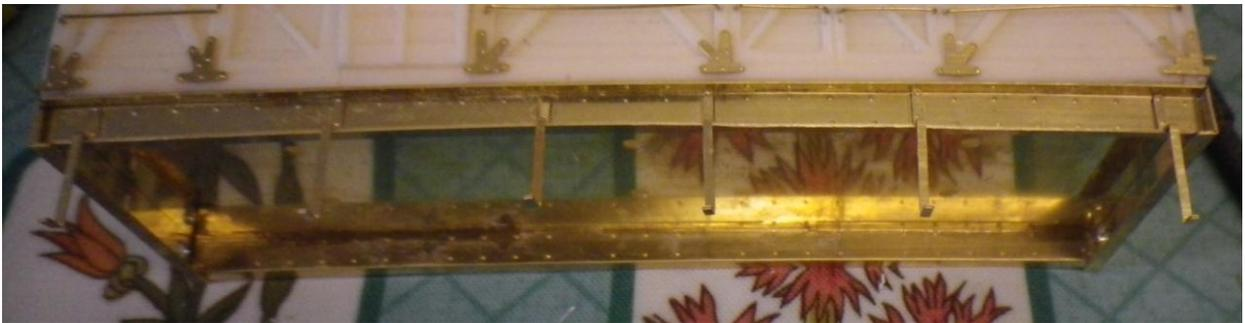
7. Now fold up and fit the running boards (part12) so that the half etched lines in the back of the running boards line up with the supports.
