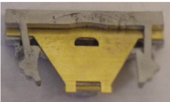
6. Then attach the brake castings (part15) to the back of the w-iron assembly.
