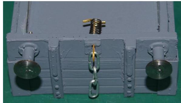
coupling hook and bend the tags over to secure the spring in place. Then fix the four buffers (part 5) into the holes in the buffer beam using two part epoxy. As shown. Repeat for the other end.
