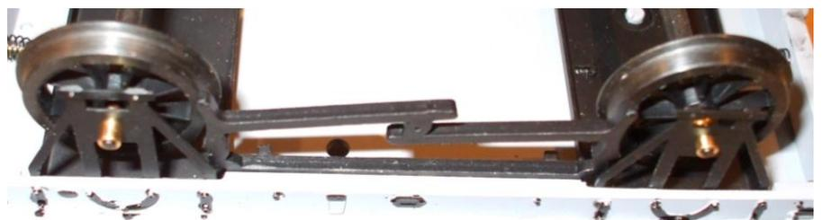
between the chassis and the sole-bar. Glue the casting into position using two part epoxy resin, this will give you opportunity for adjustment. Position the casting with care and centrally between the rivets on the sole-bar.
