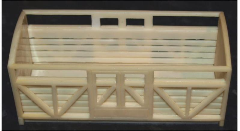
5. Next fit the etched strapping (part 5), as shown. Care is required not to get too much glue on the strapping as this could cover the strapping.
