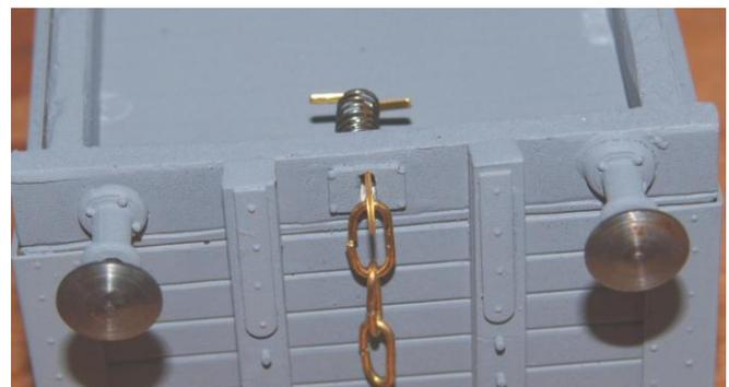
coupling hook and bend the tags over to secure the spring in place.
