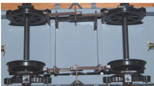
19. Glue the brake gear (part 11) onto the wagon, as shown.
