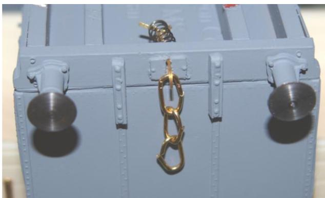
6. Next, assemble the links (part 8) on to the coupling hook (part 9) and push through the slot. Now push the spring (part
