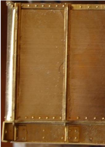
9. Next attach the support plates (part 16) for the 'T's to the sole bars.
