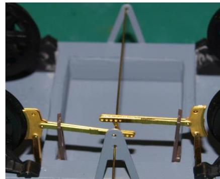
12. Fix brake lever (part25) and ratchet casting (part 26) to the outside V-hanger as shown. Repeat for the other side.
