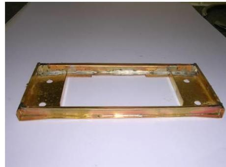
5. Next remove the buffer beam reinforcing plates (part 3) and punch out the half etched rivets and tin the back of each piece with 188C solder. Now sweat the plates onto the half etched square in the front of the buffer beam.
