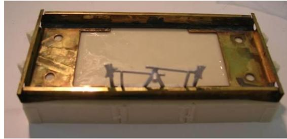
5. Drill out the w-iron castings to suit the bearings of your chosen wheels. Assemble a wheel set, 2 x W-iron's (part 7), 2 x bearing's and 1 x wheel/axle unit, do not glue the bearings into the W-irons at this stage. Again using two part epoxy resin, glue the assembled wheel set onto the sole-bars so that they are square and line up with the rivets as shown in the drawing.
