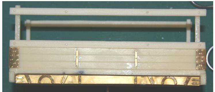
9. Next fit the two middle rails so that they are spaced evenly between the top and bottom rails.
