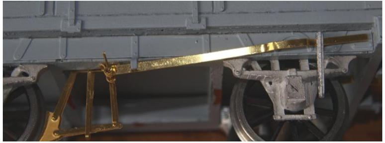
15. Next fix the brake lever (Part 18) and ratchet casting (part 19) to the sole-bar and to the out side of the brake gear pivot casting.
