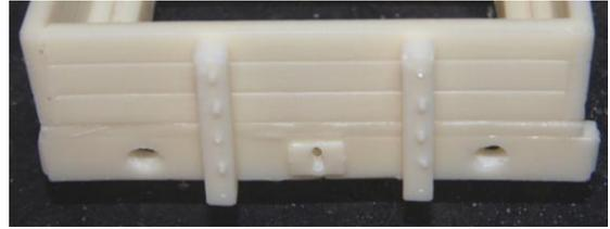
4. Next punch out the rivets on the sole bar etch (part 3) and glue to the sole bar
