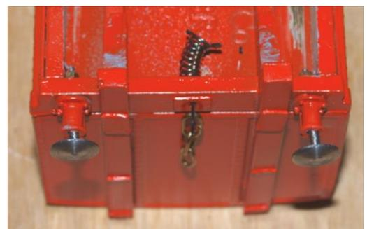
13) into the holes in the buffer beam using two part epoxy as shown. Repeat for the other end. Note the buffers have foot pads on them which go to the top
