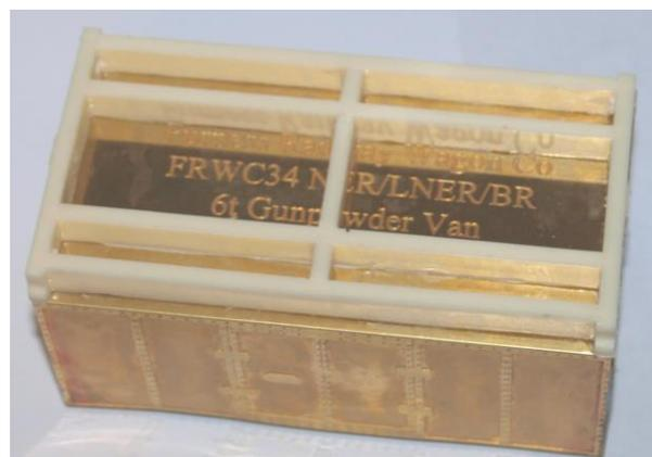
3. Attach the end beams (part 4) and end beam supports (part 5) as shown. Once secure file off the tops of the beams so that they are flush with the curve of the end.
