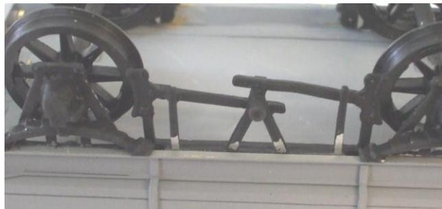
You may require chamfering the casting so that it clears the solder fillet between the chassis and the sole-bar. Glue the casting into position using two part epoxy resin; this will give you opportunity for adjustment. Position the casting with care centrally between the rivets on the sole-bar. Now glue the other brake gear casting into position on the other side. Position as per other side.
