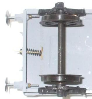
bearings into the W-irons at this stage. Again using two part epoxy resin, glue the assembled wheel set onto the sole-bars so that they are square and line up with the rivets as shown in the drawing. Note the GER used a mixture of spoked and solid disc wheels on it wagons so please refer to a photo.
