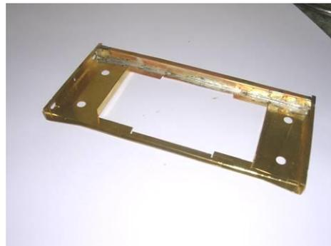
5. Next remove the buffer beam reinforcing plates (part 3) and punch out the half etched rivets and tin the back of each piece with 188C solder. Now sweat the
