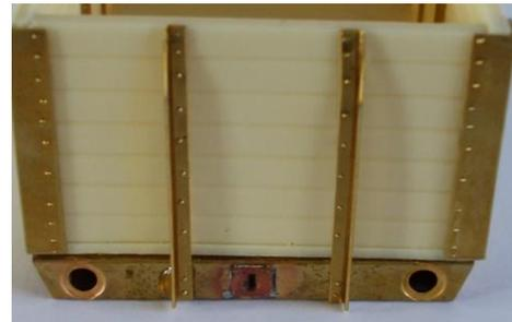
Regardless of which variant you choose you will require to punch out two the half etched reverts and either fold up the 'L' sections or solder the 'T' Sections (part 6) for the end of the wagon. Note some of these wagons were
