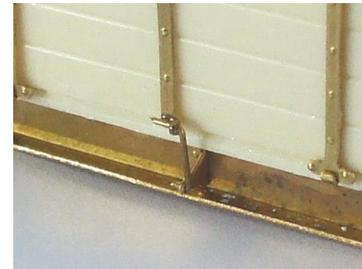
fitted with door balancers these are formed by selecting the door strapping with the lug on it and the small triangular part on the strapping etch. These need to be folded up and linked together with a short piece of wire as shown. Alternatively some wagons were fitted with conventional door stops (part 15)
