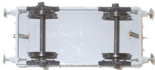
7. Next place the brake gear casting (part 13) against the inside of sole-bar and slide down into the chassis with the spigot pointing outward. You may require to chamfer the casting so that it clears the solder fillet between the chassis and the sole-bar. Glue the casting into position using two part epoxy resin; this will give you opportunity for adjustment. Position the casting with care centrally between the rivets on the sole-bar.
