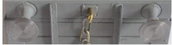
push the spring (part 10) over the back of the back of the coupling hook and bend the tags over to secure the spring in place. Then fix the four buffers (part 11) into the holes in the buffer beam using two part epoxy.
