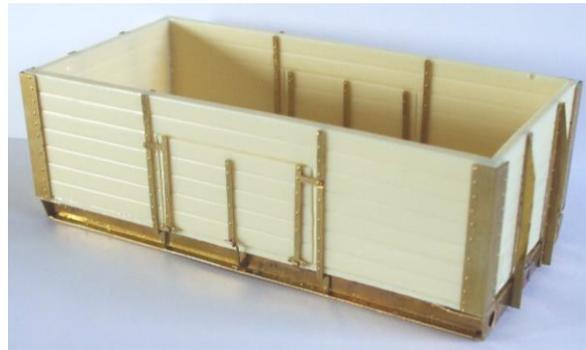
2. Next attach the strapping (part 5). Please note strapping etch will produce more than 12 different variants of the 7 plank wagon. The one illustrated is only one of these. Please consult a photograph before going any further.
