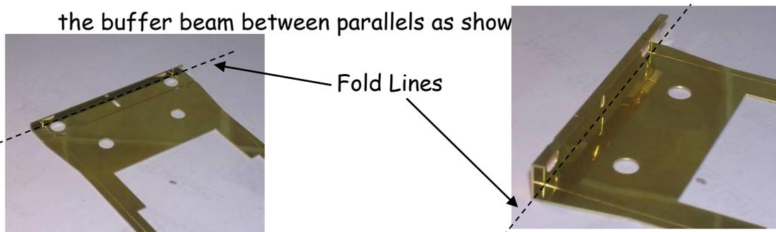
2. Next fold up the buffer beam completely as shown. Make sure that the resulting U shape is square so as to fit the sole bars. Repeat for the other end of the chassis.
