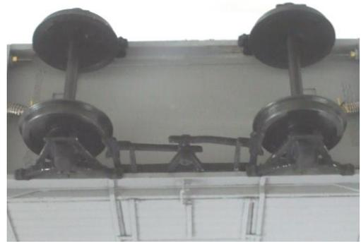
8. Next fix the brake lever and ratchet casting (part 14) to the sole-bar as shown below.
