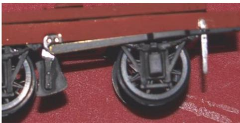
10. Next fix the brake lever (part 12) and ratchet casting (part 13) to the sole-bar and to the out side of the brake gear pivot
