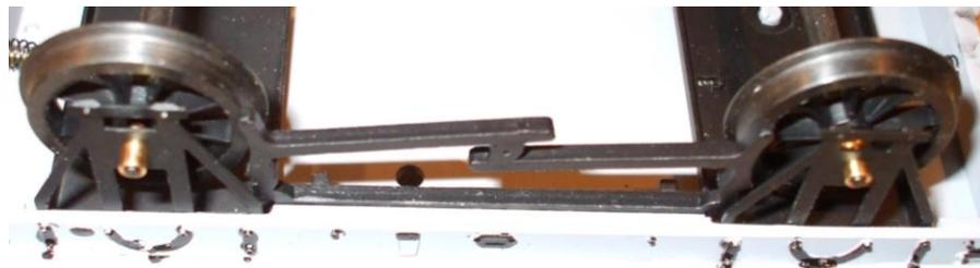
13. Next attach V-hanger (part 19) to the inside of the sole bar.
