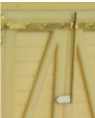
6. Then taking a piece of scrap brass from the side of the strapping etch fashion a latch plate as shown. Once this is in position attach a piece of brass wire as shown.
