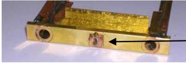
Buffer beam reinforcing plates
