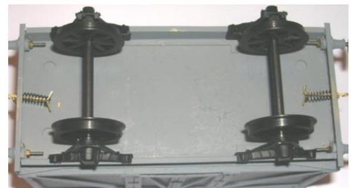
9. Place the brake gear casting (part 14) against the inside of sole-bar and slide down into the chassis with the spigot pointing outward.
