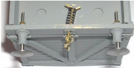
Next, assemble the links (part 9) on to the coupling hook (part 10) and push through the slot. Now push the spring (part 11) over the back of the back of the coupling hook and bend the tags over to secure the spring in place. Then fix the four buffers (part 12) into the holes in the buffer beam using two part epoxy.
