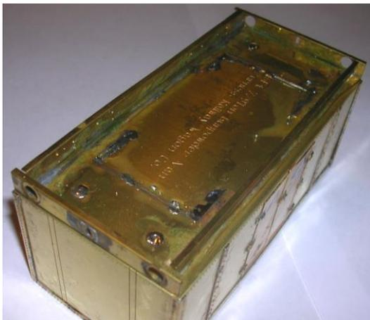
10. Solder the van top to the chassis as shown.
