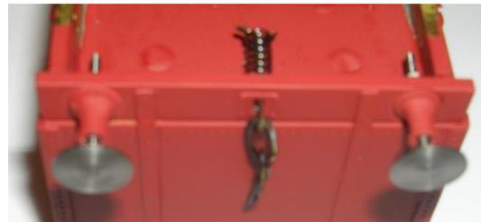
2. Drill out the w-iron castings to suit the bearings of your chosen wheels. Assemble a wheel set, 2 x W-iron's (part 21), 2 x bearing's and 1 x wheel/axle unit, do not glue the bearings into the W-irons. Again using two part epoxy resin, glue the assembled wheel set onto the sole-bars so that they
