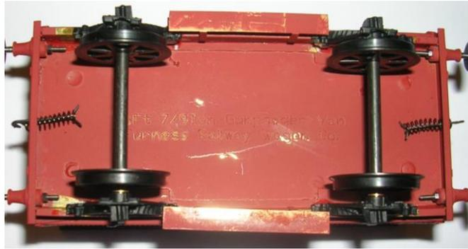
4. Place the brake gear casting (part 22) against the inside of sole-bar and slide down into the chassis with the spigot pointing outward. You may require to chamfer the casting so that it clears the solder fillet between the chassis and the sole-bar. Glue the casting into position using two part epoxy resin, this will give you opportunity for adjustment. Position the casting with care centrally between the rivets on the sole-bar.
