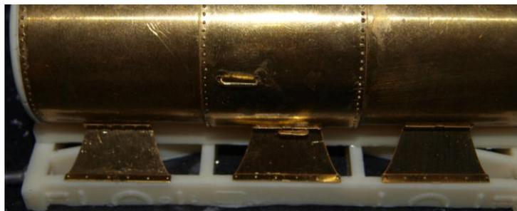
11. Assemble a wheel set, 2 x W-iron's (part 16) 2 x bearing's and 1 x wheel/axle unit, do not glue the bearings into the W-irons at this stage. Again using two part epoxy resin, glue the assembled wheel set onto the sole-bars so that they are square and line up with the rivets as shown below.
