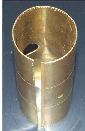
4. Punch out the rivets on the tank overlay etch (part 2) then roll in to a cylinder. Again you will require rolling bars for this task. It is also a good idea to use some card or plastic sheet when rolling to protect the rivets.
