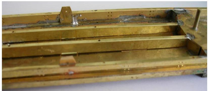
14. Using the 40thou brass wire bend up four wire supports using the template. Then solder two down struts to match the holes in the chassis assembly as shown.
