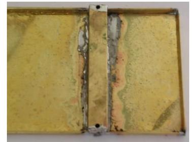
4. Next brake off part 8 (bogie supports) and fold up as shown then solder joints to give extra strength.
