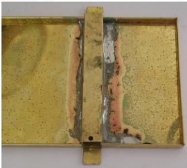
3. Solder up the bolsters onto the folded up wagon body using the tags and slots to locate them. Then fold up the last four parts of the body to form the ends of the bolsters and solder into positions
