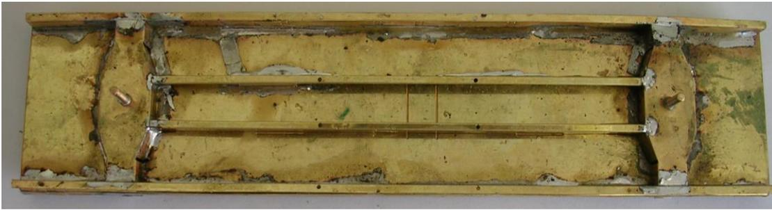
11. Brake off parts 11 (buffer beam plate), 12 (Buffer beam detail) and 13 (coupling hook plate) from the etch and sweat them together.
