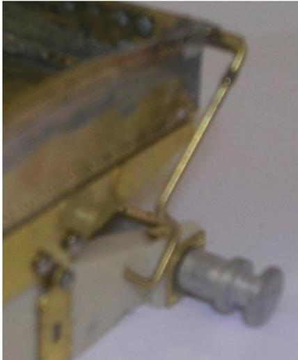
15. Next fit the bar into the tube on the tank and scribe a curved line on each end of the chassis. 5mm above the bottom of the chassis draw a line to cross the curved line. Where these lines cross drill a hole into the chassis on that line to act as a pivot.
