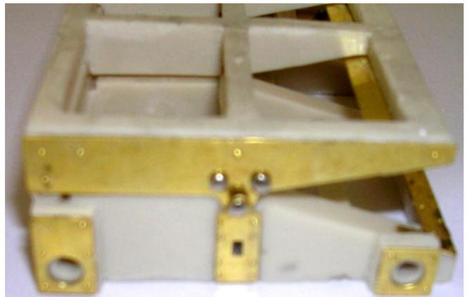
11. Next, assemble the links (part 20) on to the coupling hook (part 21) and push through the slot. Now push the spring (part 22) over the back of the back of the coupling hook and bend the tags over to secure the spring in place. Then fix the four buffers (part 23) into the holes in the buffer beam using two part epoxy as shown. Repeat for the other end.
