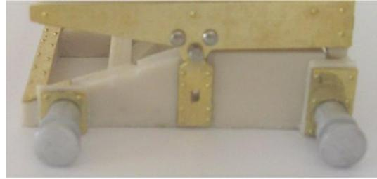
12. Take the long straps (part 24) and punch out the half-etched rivets and bend up and fit. They should fit half way between the buffer beam and the centre beams as shown. Repeat the process for the other side using the shorter straps (part 25) as shown.
