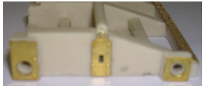
7. Next take the top casting (part 16) and fit the side reinforcing beam (part 17) into the slot. The slot may require a file running across it to clean up the edge.
