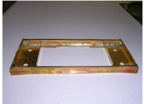
5. Next remove the buffer beam reinforcing plates (part 3) and punch out the half etched rivets and tin the back of each piece with 188C solder. Now sweat the plates onto the half etched square in the front of the buffer beam.
